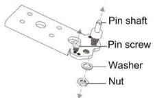
8. Insert the pin screw into the right hole and insert the pin shaft into the left hole on the lower hinge,, then secure the shaft with the washer and nut.
