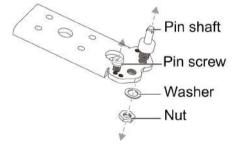
8. Insert the pin screw into the right hole and insert the pin shaft into the left hole on the lower hinge,, then secure the shaft with the washer and nut.
