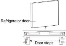
11. Install the refrigerator compartment door.12. Move the door bushing from the top right side of the refrigerator door to the top left side of the door. And move the left hole cover to the right side.
