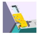
10. Take out the top left hinge cover, connect it with the wiring harness, and install them on the cabinet.
