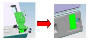
3. Screw off the three bolts fixing the top box cover on the left side, remove the box cover, take the wire harness out of the hole, and transfer the door shaft sleeve from right
