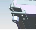
7. Remove the door stopper and door closer, take out the door closer from the accessory bag, and install it on the left side of the door.
