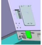
4. Lift up the refrigerator door by 50mm to remove it.
